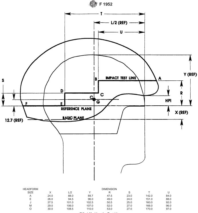
FIG. 1 Marking the Test Line
